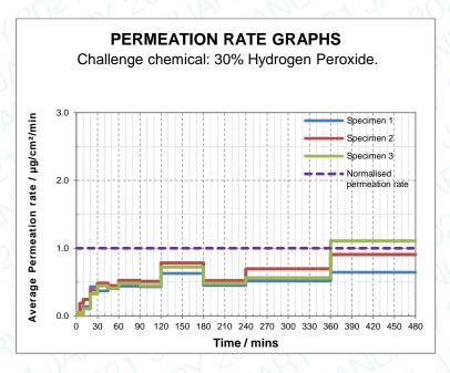
Hydrogen peroxide is determined by discrete sampling; therefore the permeation rate graph is not a smooth curve.
